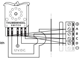
Pic. 1. How to connect the display with a BCD Preselector BCD.
