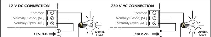
**INFORMATION ABOUT THE OUTPUT.** During the operating mode and according to its load, it could happen a fluctuation or an incorrect working of the output. In such case, you have to install an anti-spark circuit between both contacts of the used relay, as it is indicated on the schedule.
