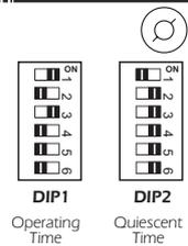
**Note.** To allow the module to recognise the timing value change on DIPs, you have to reset the circuit.
