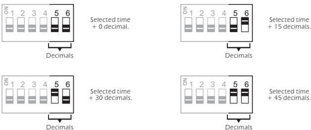
**If you don't select any time on both DIPs, the module would identify the selection as wrong and wouldn't start the timing.**
